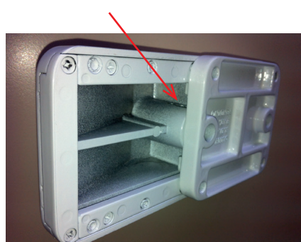
Position of push-button on Thule Door Lock
